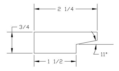
DESCRIPTION 103 RAIL CLIP FLAT BOTTOM BOLT MAT'L WEIGHT BOLT GAGE TYP SPACING REV 24" .70 lbs A36 N/A N/A 0 SCALE TOL. PART NO. RCF103000 NONE +/-.030
