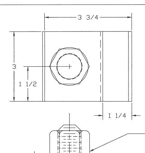
SINGLE HOLE CLAMP WITH WELDED
