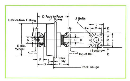
Flange Mounting Box FM-1 is available for use on the 1 through 8 ton wheel assemblies using tapered roller bearings.
