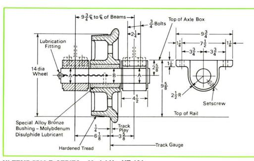
The Irwin 3 through 7½ ton Stub Axle 550°F. Wheel Assembly includes:
